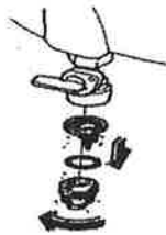
Fuel Filter Element Removal
